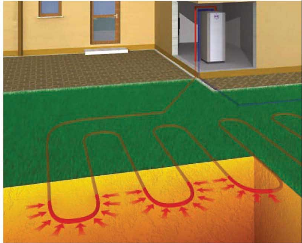
Diagram of earth-water heat pump principle, a horizontal ground collector
